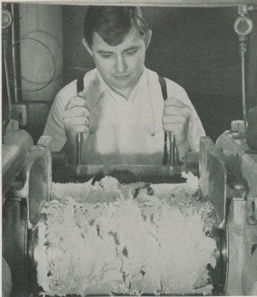
The machine above kneads pigment, filler and plastic base together in the preparation of diallyl phthalate molding powder. Below, the press reveals characteristics of a rubber blend in the development of Dutrex plasticizers.
