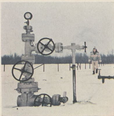
Marking the discovery well at the Bonnie Glen field near Edmonton is this "Christmas tree" that juts unexpectedly out of a mantle of snow.
