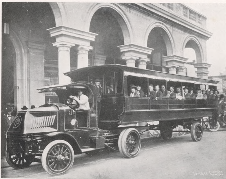
Three-and-a-half-ton tractor truck and five-ton Texas trailer with bus body having seating capacity for one hundred persons, built by The Texas Wagon Works, Houston, Texas, for The Texas Company's Morgan City, La., Shook Mill, to be used for transporting employees to and from the mill which is located about three miles out of Morgan City.
