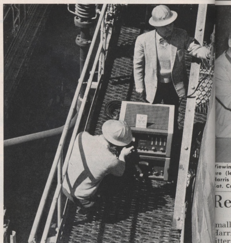
Dr. T. B. Metcalfe (standing) and Dr. R. H. Hunt of the Research Lab use a portable monitor to study the flow pattern in a cracking unit. The passage of gamma through the unit indicates the pattern.
