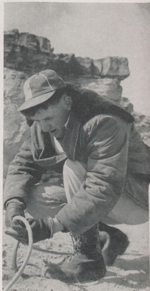
4. After digging holes with a tool called a post hole digger, McKenzie "plants" jugs and connects them to cables like this one, which run to the seismograph truck stationed nearby.
