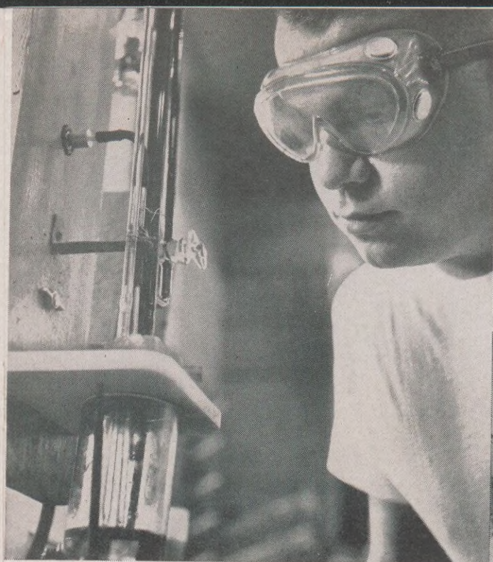
Production of versatile synthetic glycerine from petroleum requires precise control to insure that it is more than 99 per cent pure. One control test conducted during synthesis is a water analysis of samples of dilute glycerine being conducted, left, by Operator L. L. Born. Tests are conducted throughout the manufacturing process.
