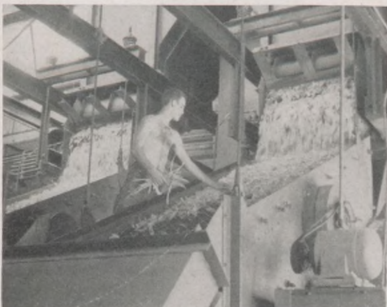
> A final phase of papermaking is "calendering," right. Near-finished paper goes through batteries of steel rollers. These give paper the desired surface.
