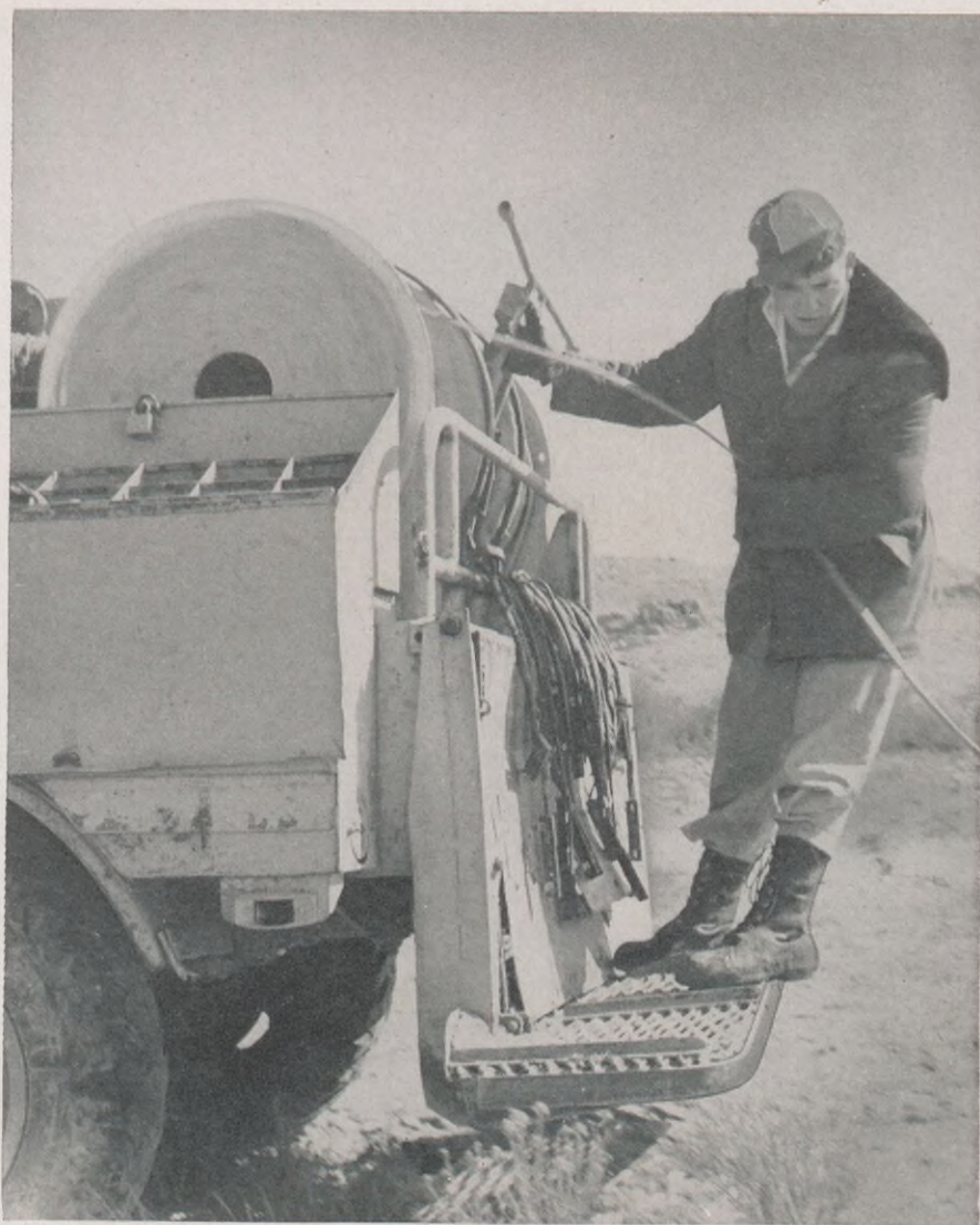
6. In the field, McKenzie works as a team with another jughustler. Part of the time, he reels out cable from the back of a recording truck, above, while his partner plants the jugs and connects them to cables. Jughustlers must work fast, following lines determined by the party's surveyors.
