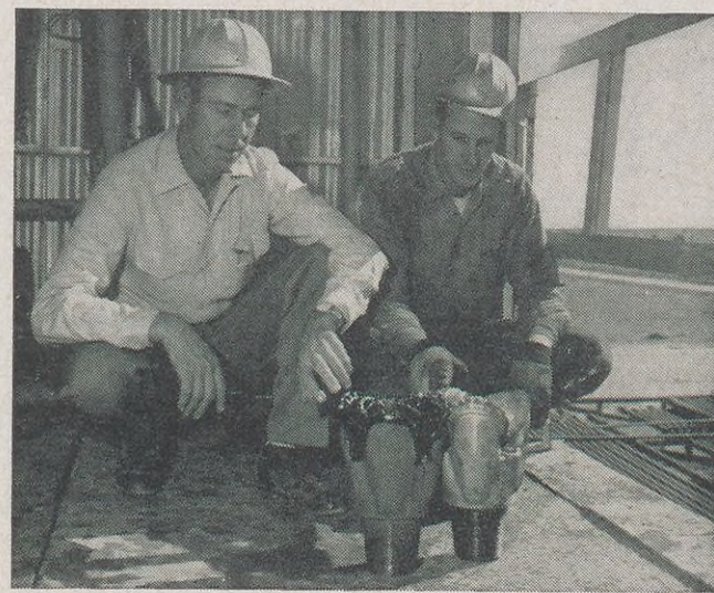
On the rig floor, Drilling Foreman R. B. Flournoy (right) and Joe compare a new drilling bit (left) with a worn one that had to be brought up and replaced.
