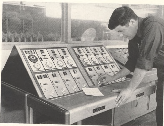
Central feature of Texaco's newly opened River Rouge, Michigan, lubricating-oil blending plant is an electronic control console, above, that enables a technician to mix as many as six additives and base oils at a time. The multimillion-dollar, high-speed plant will blend and compound for industrial and automotive uses more than 40 types of Texaco products, including Havoline and Texaco Motor Oils, and Texamatic Fluids.
