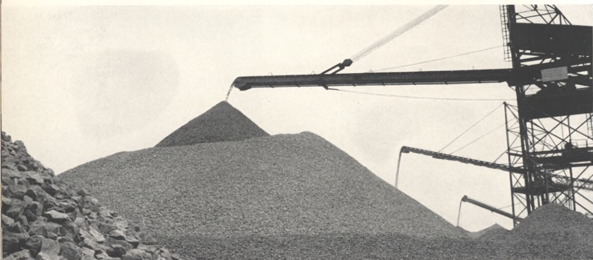
Pyramids of crushed rock rise below jutting snouts of conveyor belts. Side-dump trucks will carry stone to nearby concrete-mixing plants.
