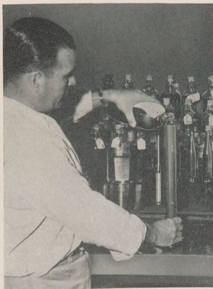
12. Meanwhile the samples of crude, already at the control laboratory, are being tested for gravity and for bottom sediment and water. Here Tester F. E. Dufresne pours a sample into a glass graduate for a gravity check.
