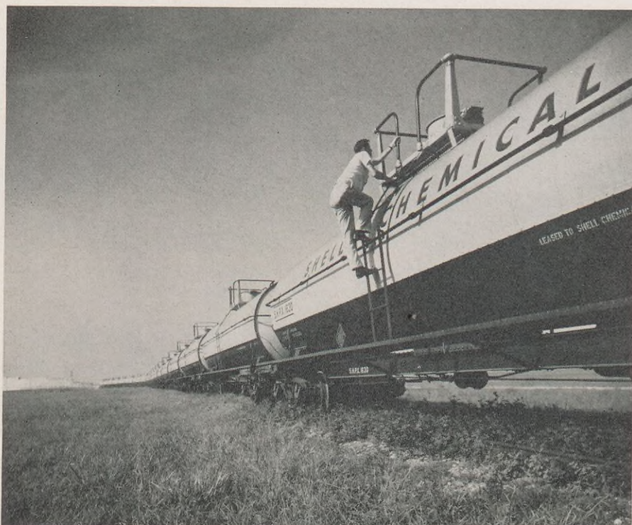
Ethyl chloride, the antiknock fluid for automotive and aviation fuels, is shipped from Shell Chemical Corporation's Houston Plant in pressure tank cars such as the ones shown above.
