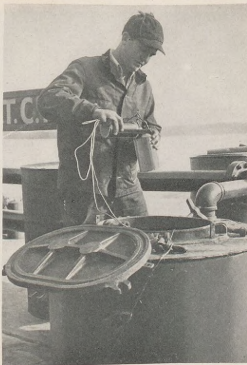
7. Using a "thief"—a sampling device—Dock Helper Stanley Adams takes a quart of crude from each compartment for laboratory testing.
