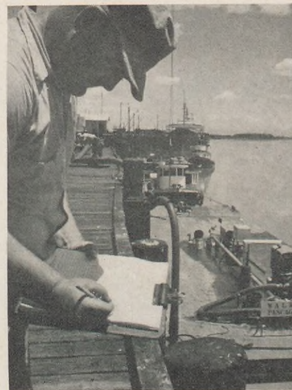
11. Pumping underway, the dockman fills out a barge unloading report, noting soundings of each compartment and samples taken.
