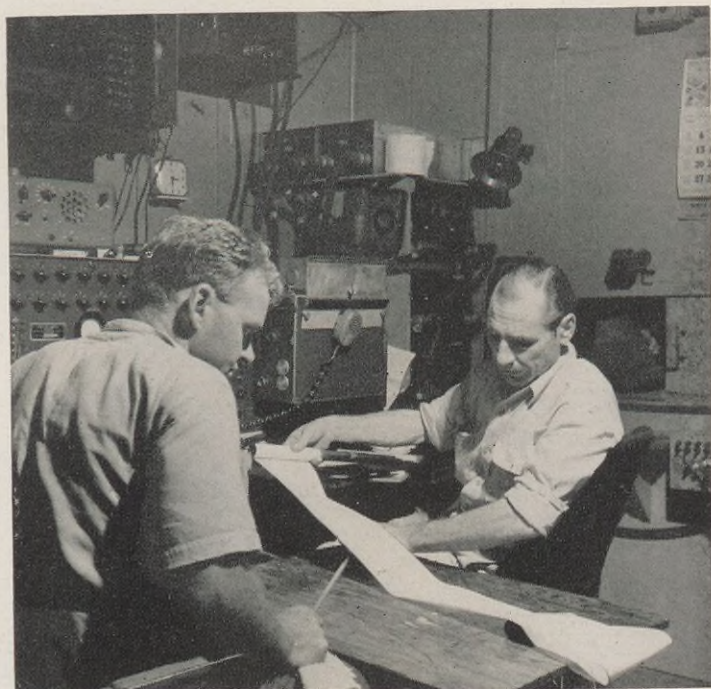
9. Two operators of the recording instruments on the instrument boat, above, examine the long strip of film on which the shock waves reflected from the strata beneath the Gulf is recorded. It is similar to land-based seismic film.
