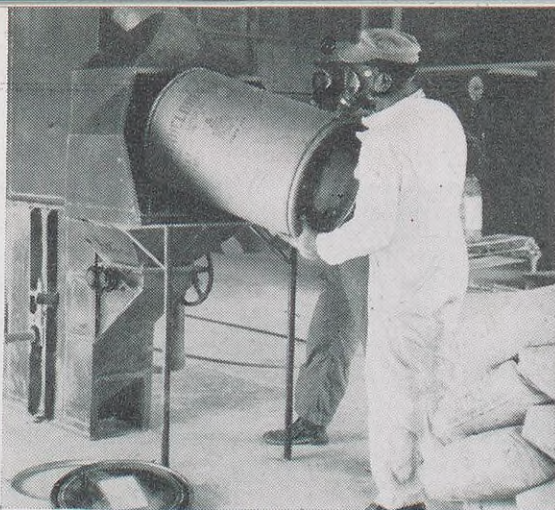
Shell Chemical Corporation's dieldrin insecticide is mixed to field strength here in a formulating company's plant.
