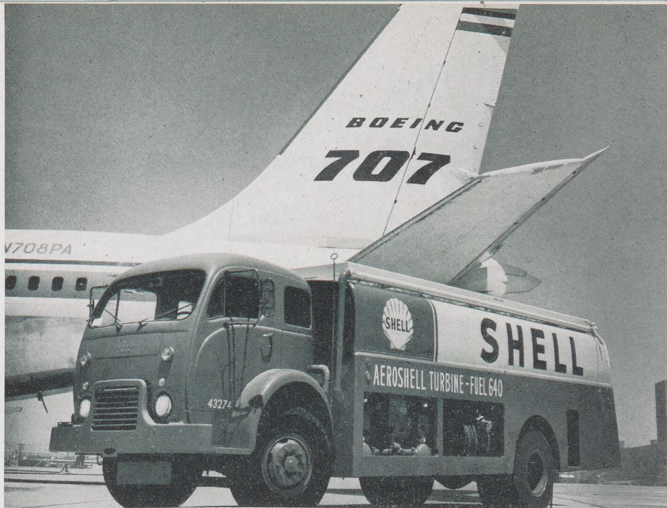
Shell Oil Company engineers have designed special fuel trucks for use in jet-age fueling operations. The trucks have a capacity of 5,000 to 8,000 gallons and are equipped with special filters and dehydrators to keep the turbine fuel free from contaminants. The trucks will pump fuel at rates up to 600 gallons per minute.
