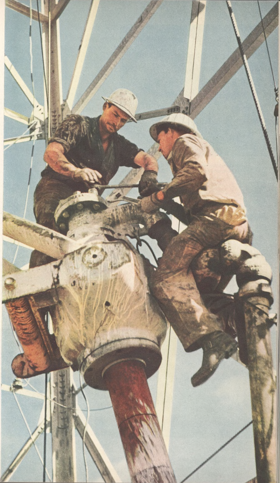
High above the blue Gulf, roustabouts connect the rotary hose to the swivel in the rigging-up. Drilling fluid flows through this hose to the swivel, then down the drill stem to the bit.
