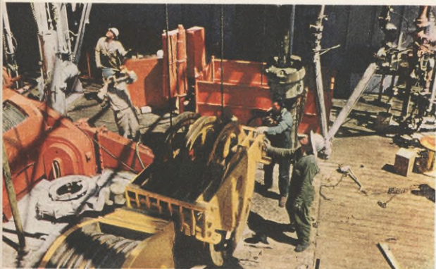
The crew strings up traveling and crown blocks before spudding in a tidelands test.
