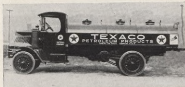
New designs in trucks to be used in Northern Territory. One, a 600-gallon 3-compartment Mack tank truck with can racks; the other a 3 1/2-ton 1,000-gallon 3-compartment tank truck with can racks.
