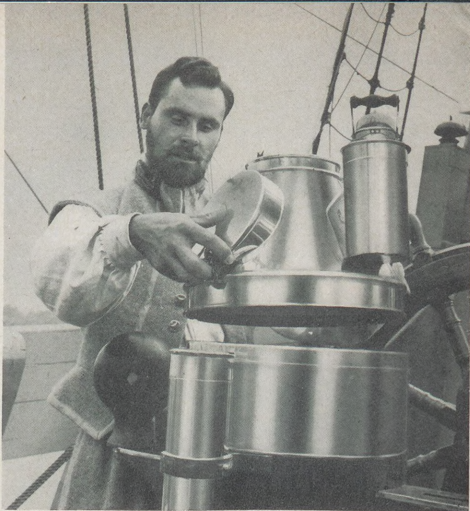
Here Ford puts the brass top, which he polished, over the compass. The top has a built-in oil lantern, on right.
