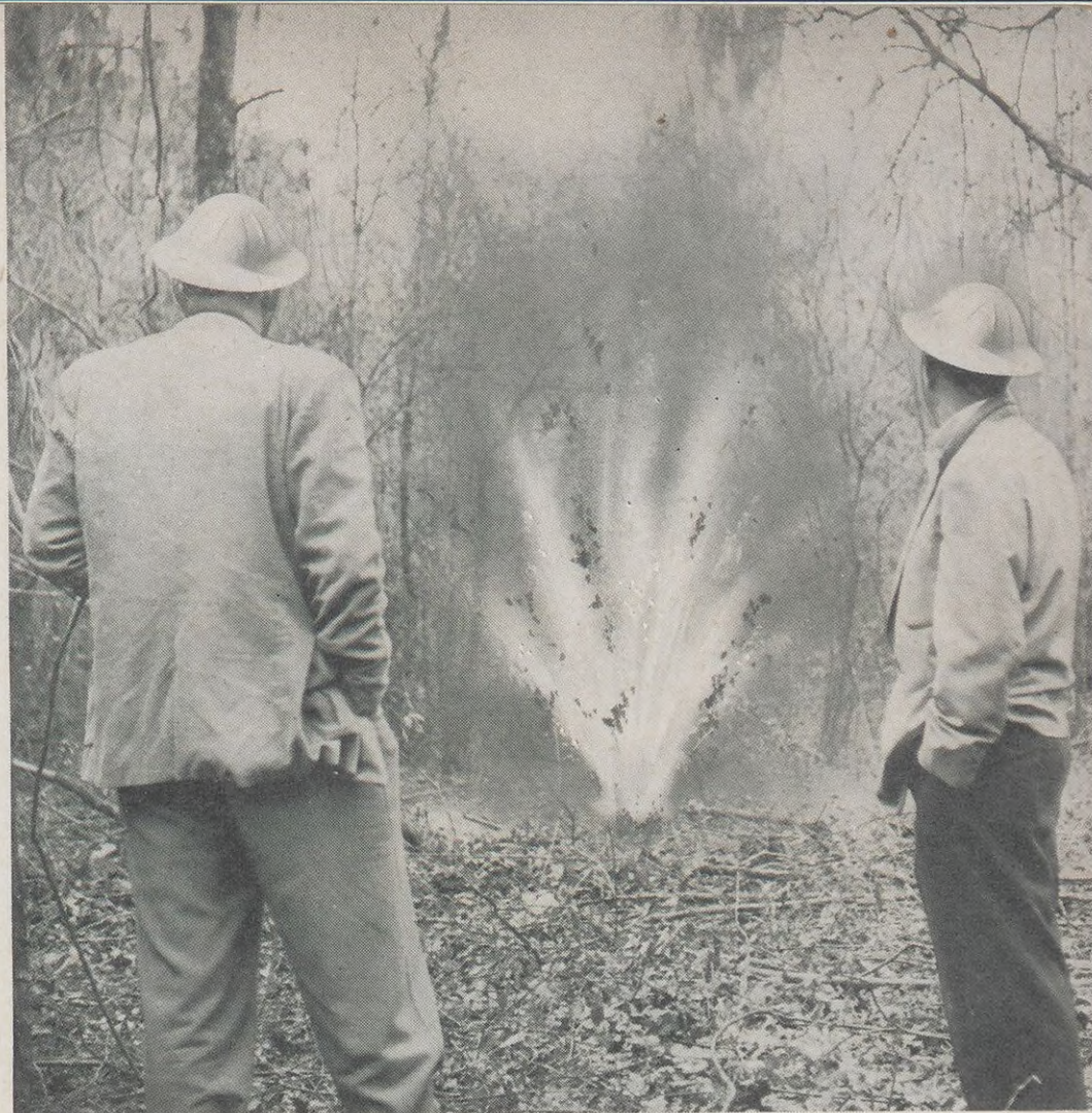
V. E. Liles, left, and J. T. Hartman watch the spray of mud and water caused by the seismic shot, the sound waves of which are recorded by delicate instruments. The shots produce data to help map the sub-surface earth structures for further study.
