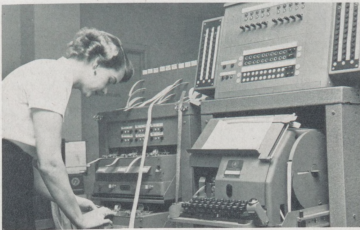
Mrs. Elaine Halliday, Teletype Operator in Shell's San Francisco office, sends a message over a transmitter-distributor machine. This complicated instrument transmits messages to different Shell locations which are selected on the push-button board on the right.
