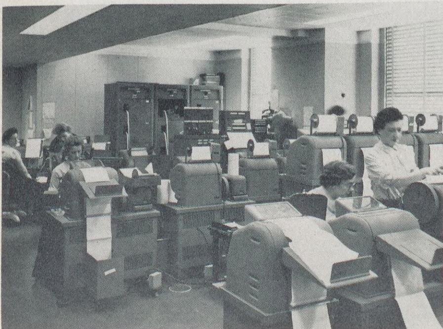
The hub of Shell's teletype system is this room in Head Office. Teletype messages are not only sent and received here, but also are relayed between points which are not connected by direct wire.
