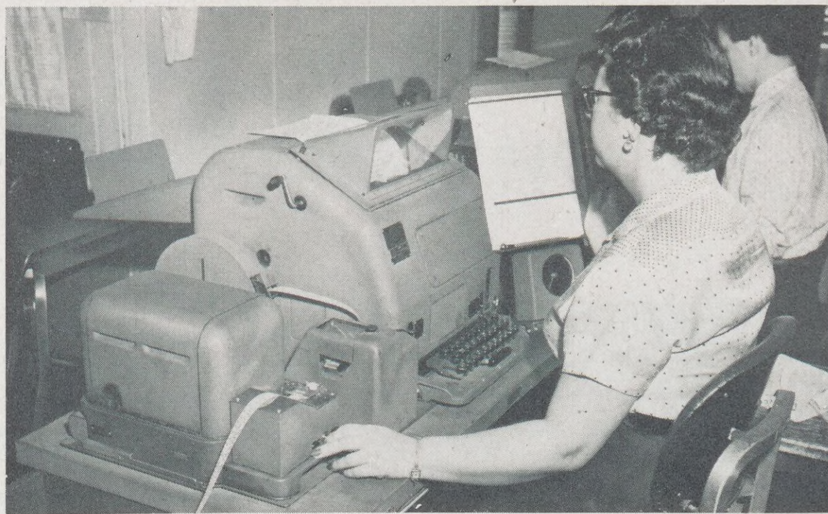
Teletype Operator Selma Zober starts a message on its way from the Head Office communications room. She prepares the teletype message on a perforated tape which is then fed into a transmitter and simultaneously received at the intended destination.
