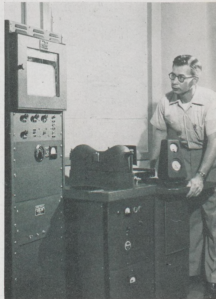
An X-ray diffraction apparatus also was used in analyzing the crystal structure of various spark plug deposits. Above, Laboratory Assistant E. V. Kepner operates the unit.
