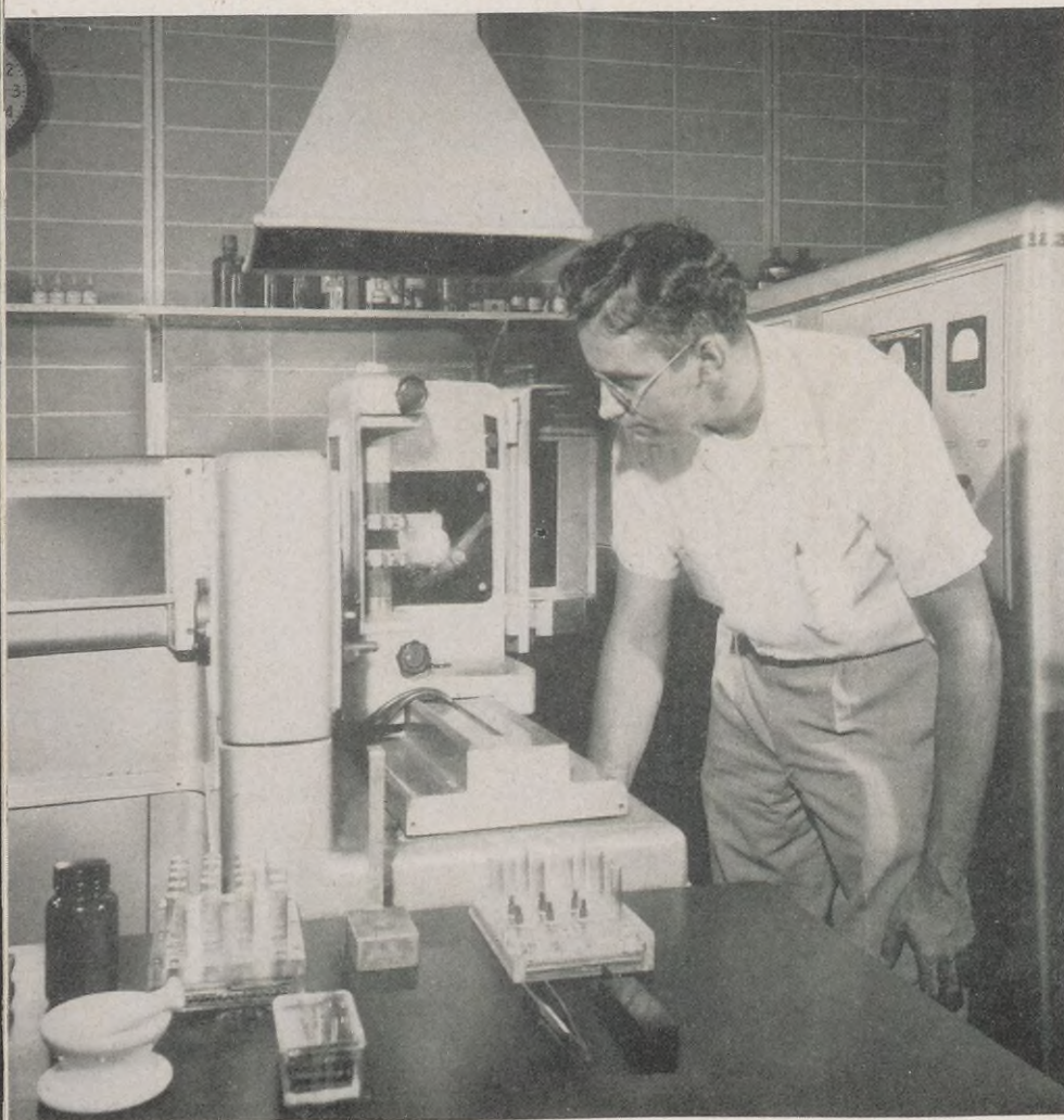
Unusual instruments such as the one shown here are effective tools in the search for more information about oil. Chemist R. J. Grabowski is "activating" a sample in an emission spectrophotograph, which analyzes petroleum, minerals and other substances.
