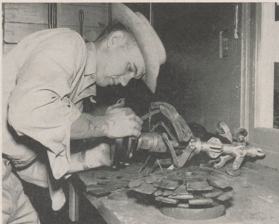
Andersen replaces rubber discs on a go-devil at a pump station repair shop. In the foreground are worn rubber discs, used on a cleaner in a pipe line of varying diameters. Designed by Shell engineers, the notched discs contract as a cleaner enters smaller pipe.
