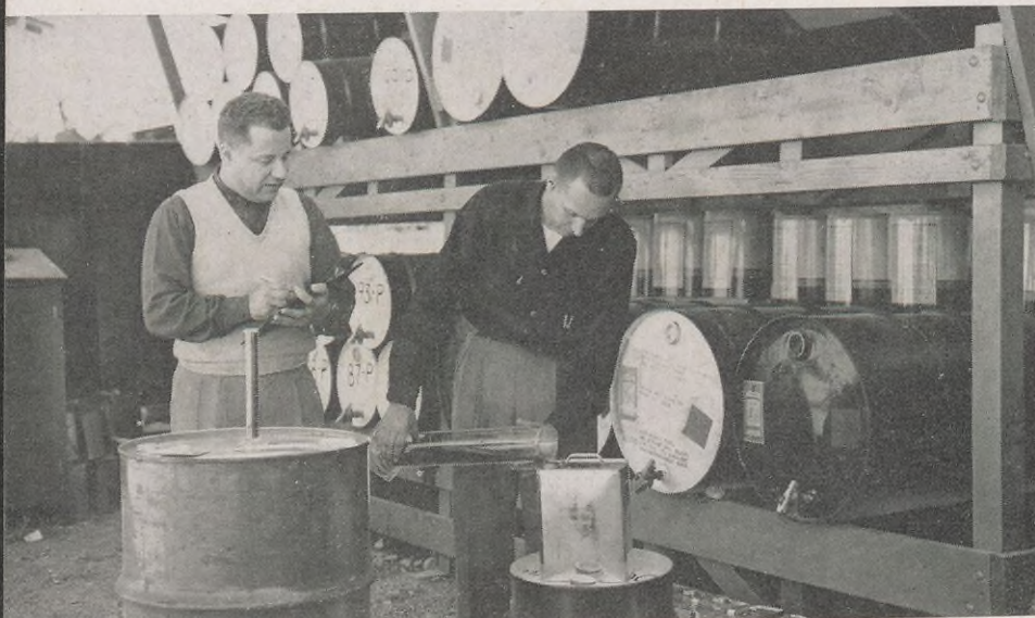
Phalen, left, and J. E. Cox, Products Application Department Engineer, blend a reference fuel of known octane number to be used to check the knock rating of the 1956 model automotive engines in the test. Each motor has a different rating.
