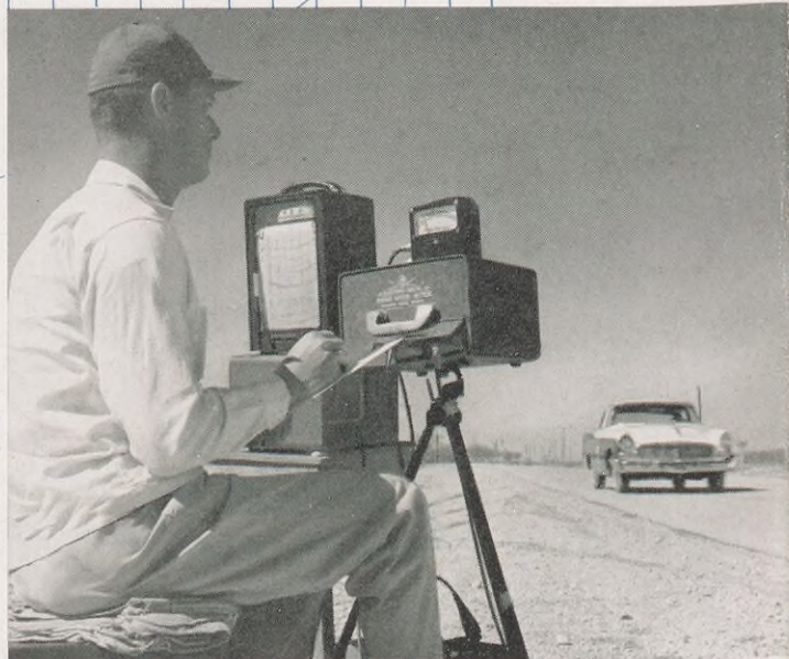
A test car zooms down the road at San Antonio, Texas, during one of the tests of gasolines in 1956 automobiles. The radar instruments chart the car's speed and give its acceleration time.
