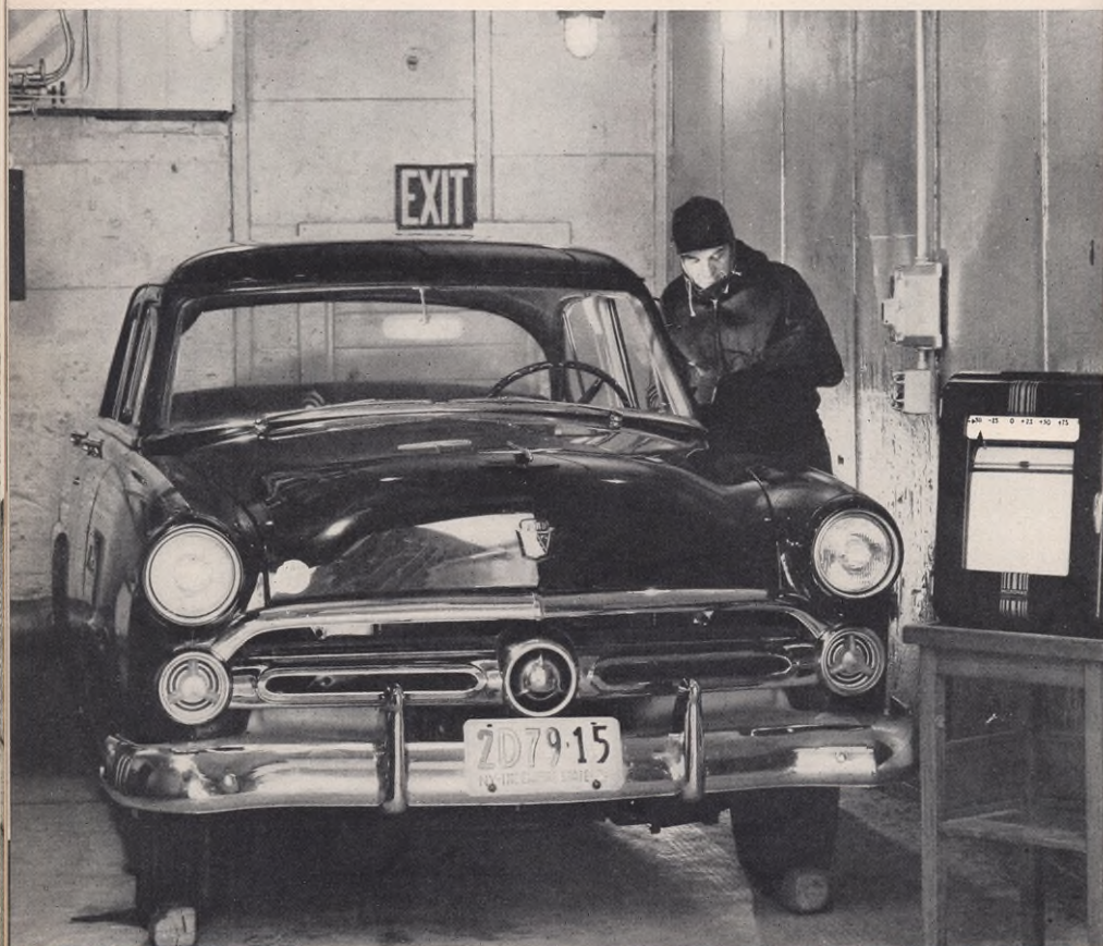
BEACON, N. Y.—FUELS AND LUBRICANTS UNDERGO SUB-ZERO TESTS IN FROST-FREE COLD ROOM
