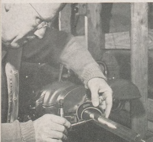
Gunsmithing requires precision machine work. A micrometer measures a part to its nearest half-thousandth of an inch.
