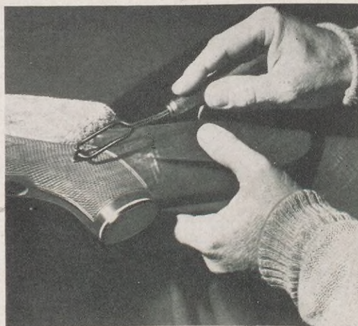
Stock is checked for decorative purposes and to give it better grip. A meticulous process, checkering takes infinite patience and about two days' work.
