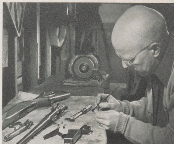
Hand-fitting a metal part in the trigger mechanism, as Heid is here, is an exacting job.
