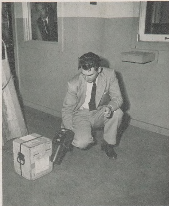
Chemist V. P. Guinn, with an ionization chamber, monitors an incoming shipment of radioisotopes, determining the radiation level outside the package before it is sent to the laboratory.
