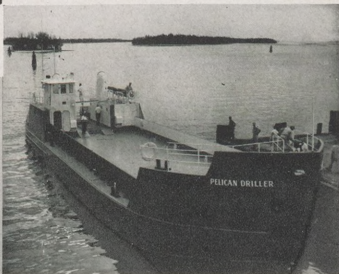
Four special vessels serve the offshore platform when it is drilling. Above is the Pelican Driller, which hauls drill pipe and heavy equipment. Other boats which are smaller, carry personnel and light supplies.
