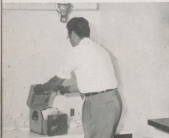
Chemist C. D. Wagner, wearing gloves, opens the outer container of the radioactive shipment. Lead bricks in front reduce the radiation.
