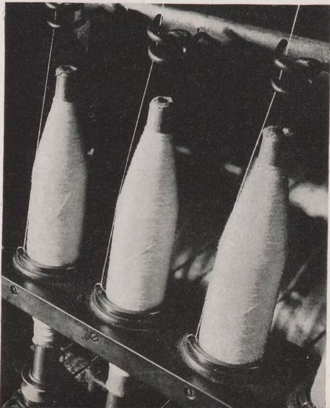
Cotton Ring Spinning Spindles run at speeds from 5,000 to 12,000 R.P.M.
