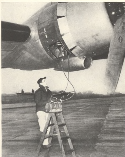
This unit, removed from within the nacelle for demonstration purposes, carries a Texaco developed cold-starting fuel which slashes starting time in sub-zero temperatures
