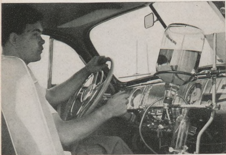
Demonstrated in C. F. Zimpel's automobile (above) is the fuel storage and feeding system required by Mileage Marathon rules. The measured quantity of gasoline is carried in the driver's compartment and fed to the engine through a temporary line.
