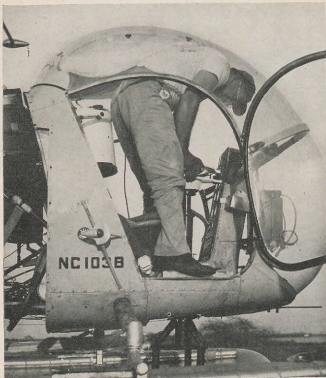
Gravity Meter Operator P. E. Duplantis releases the tripod, carried between the pontoons of the plane, and plunges it firmly into the waterlogged earth, after the helicopter has landed on a designated section of marshland.
