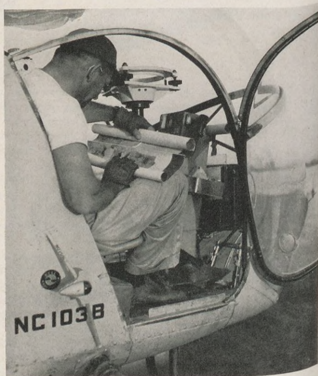
When the gravity observation has been taken, the meter is removed and placed in its carrying position and the tripod is retracted. The operator then examines aerial photographs to determine the course for the flight to the next station.
