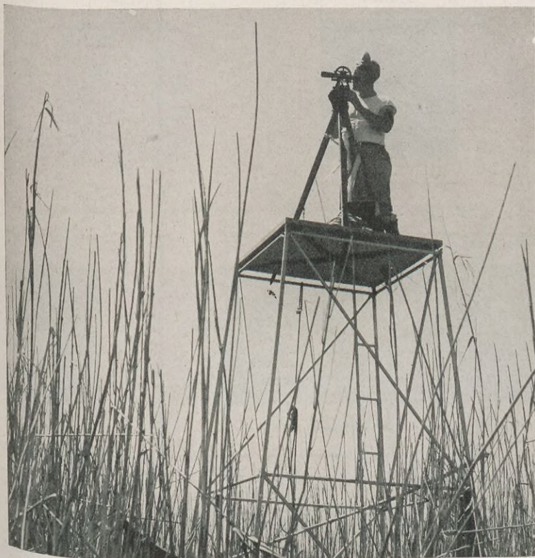
Surveyors, flown in by helicopter to determine gravity observation positions, use folding, 12-foot aluminum towers to raise themselves and their transits above the tall reeds and marsh grasses.
