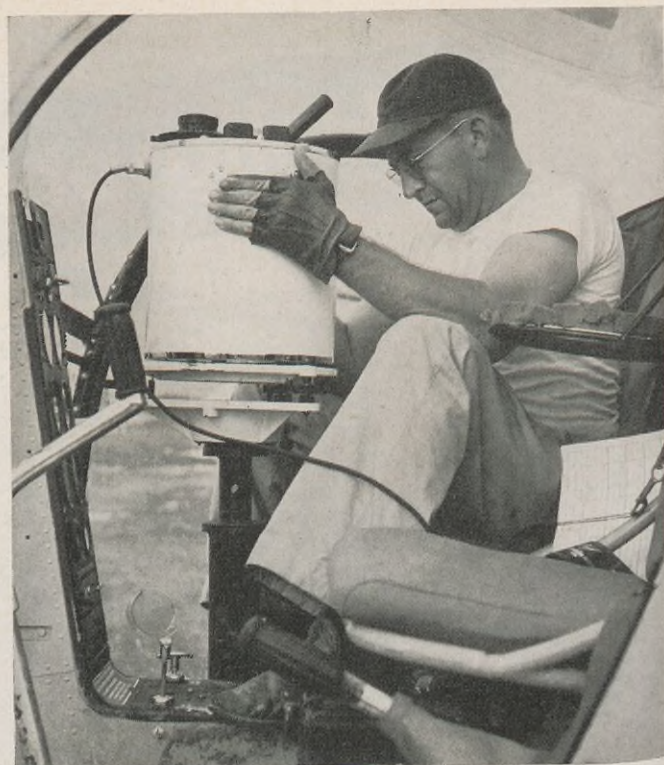
The sensitive gravity meter is then removed from its special carrying attachments and placed on the leveling head of the tripod. A storage battery, used to supply current to the gravity meter, is carried under the pilot's seat.
