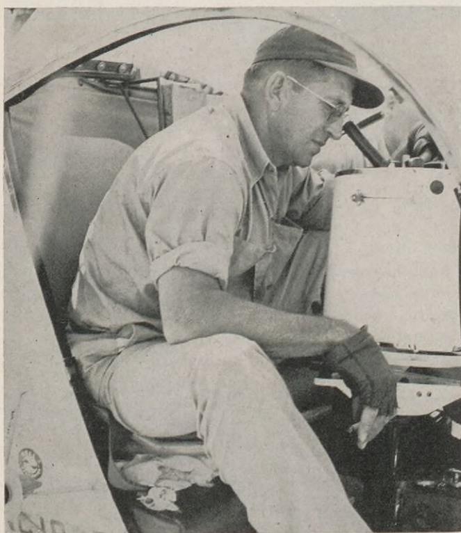
Although neither the gravity meter nor its tripod touches the helicopter while Duplantis takes his reading, the motor and rotor blades must be completely stopped as the vibration shakes the marsh, preventing the meter from coming to rest.
