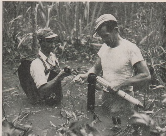
A dynamite charge is about to be lowered into the hole and set off, to create elastic waves which will be recorded on the seismometers.
