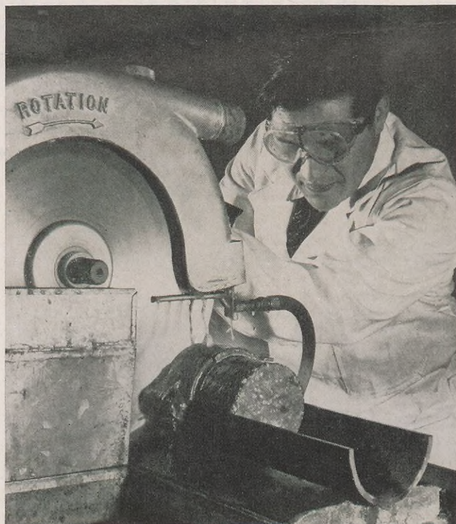
Much as a butcher would slice bologna, a technician cuts a sample core into thin slices for study. Though the core contains hard, solid rocks, the cutting edge slices through in a matter of seconds, leaving the core structure unaltered.
