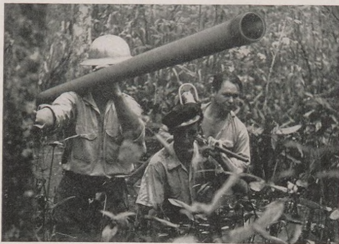
With the seismometers planted, the next job is to prepare the casing through which a shot hole will be made to hold the dynamite.
