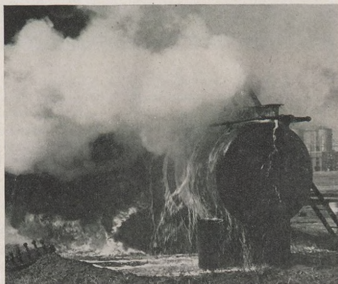
Enveloped in this mass of flame and smoke is a 10 x 6-foot vessel filled with gasoline. The sprinkling system installed on the vessel, along with fog nozzles, extinguished the fire in the short space of one minute and twelve seconds.
