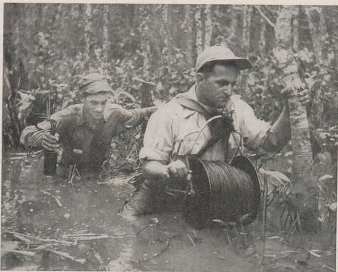
When the proper location is finally reached, the crew sets out the seismometers, which are connected by cable to the recording unit.
