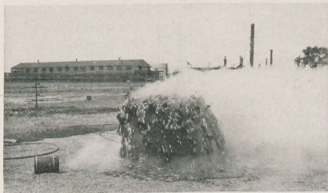
The right way and the wrong way to extinguish an asphalt fire. At left, when water is poured on the fire the asphalt boils over. At right is shown the extinguishing action of low velocity steam when used on the same type asphalt fire.
