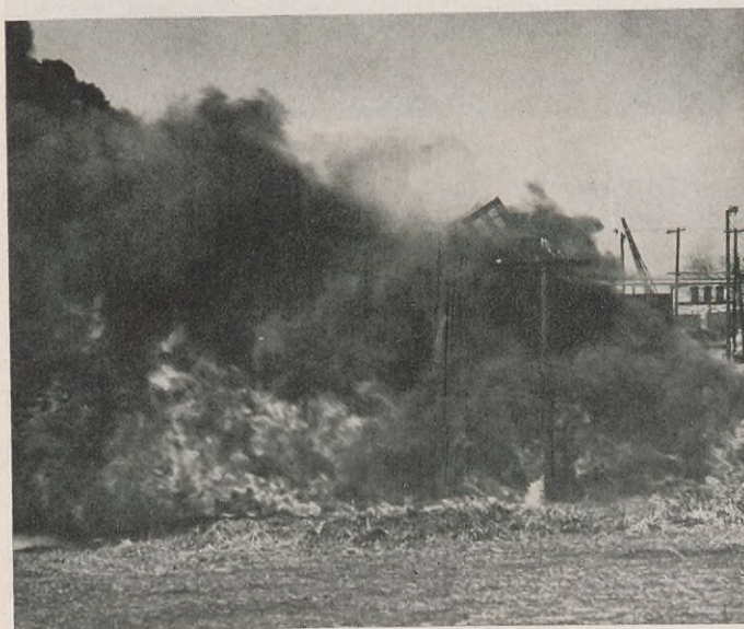
Enveloped in this mass of flame and smoke is a 10 x 6-foot vessel filled with gasoline. The sprinkling system installed on the vessel, along with fog nozzles, extinguished the fire in the short space of one minute and twelve seconds.
