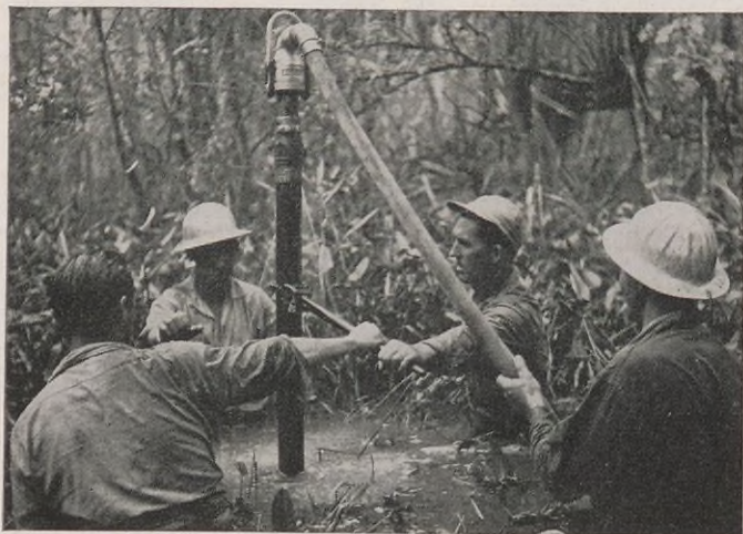
The shot hole is made on the swamp bottom by pumping water at high pressure into the casing as it is wrenched down into the muddy floor.
