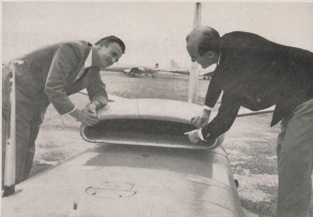
Engineer Frame-Thomson, right, shows the humped air scoop in the flying lab's back to D. C. McMacken of the Products Application Department. Air rushes into the scoop, through a turbo-jet engine, and out the vent in the tail assembly, as shown below, at left.
