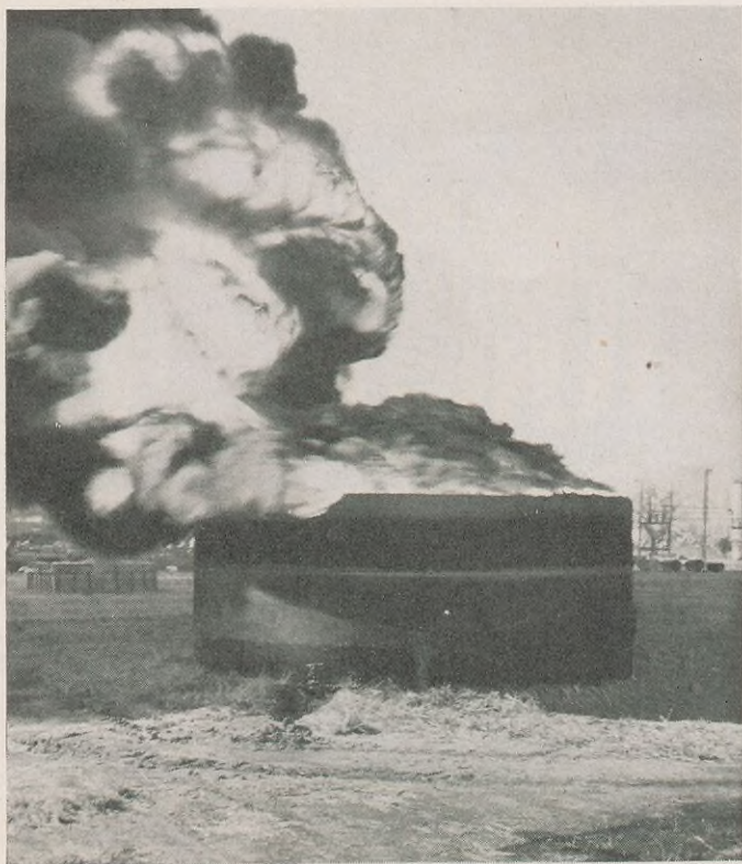
< Fog was used to extinguish the blaze on this twenty-foot diameter tank. It took only one minute and nine seconds to put out the fire with the use of two 1 1/2" fog nozzles. Selection of the correct extinguishing agent for each type of fire is emphasized in the course.
