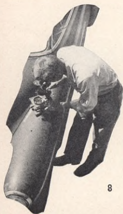
WITH microscope on car fender, Texaco Geologist examines core sample of rock brought up from bottom of drilling well for indications of oil
