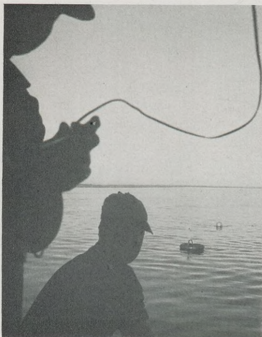
5. The shooter prepares to set off a suspended charge (hung from the toy balloon beyond the buoy). This technique is sometimes substituted in offshore operations for the shot hole system.
