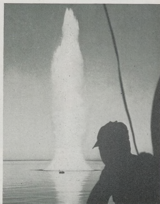
6. As the shooter pushes the button, contact is made and the suspended shot is detonated, causing a geyser of water to shoot 100 feet into the air some distance from the boat.
