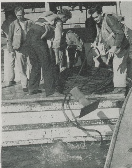
2. Seismometers, attached at 200-foot intervals to a cable run out from the instrument boat, are sunk on the ocean floor along the line marked by flags previously planted from the survey boat.
