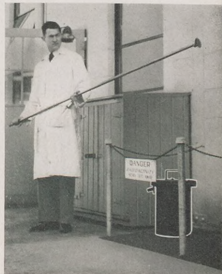
Hazard: Radiation. Prevention: A lead-lined well is used to store radioactive gears used in lubricants research.
