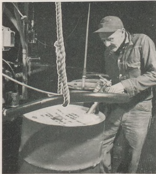
Hazard: Over-exertion. Prevention: Nothing more than a rope loop. But it holds up the heavy hose in a drum filling operation, and it also prevents spilling.
