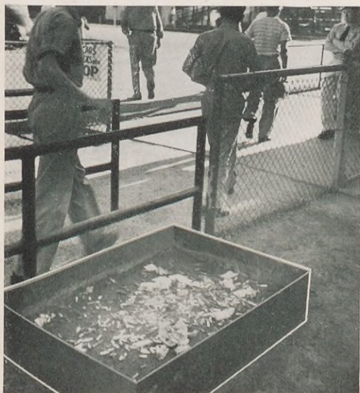
Hazard: Fire and explosion. Prevention: Receptacles for depositing cigarettes before entering Shell refineries are standard equipment.
