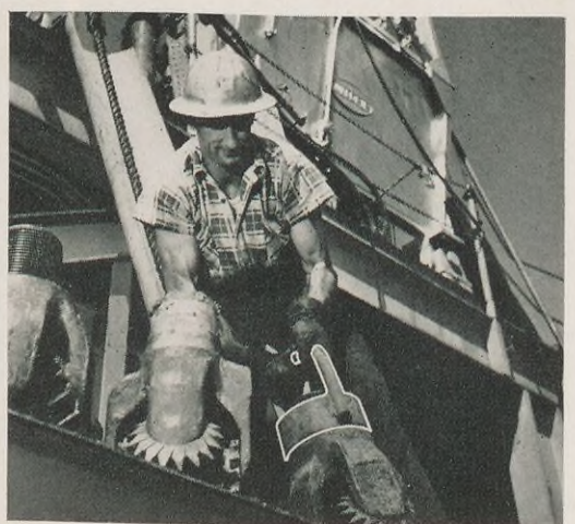
Hazard: Over-exertion and falling objects. Prevention: This simple bit handling tool, devised by Shell employees, makes lifting heavy bits easier and avoids toe-smashing slips.
