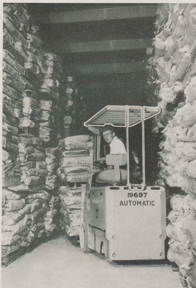
Hazard: Falling Objects. Prevention: This fork lift moving pallettes of sacked chemicals in a plant warehouse has a protective grid over the operator to stop or deflect sacks that might possibly fall.
