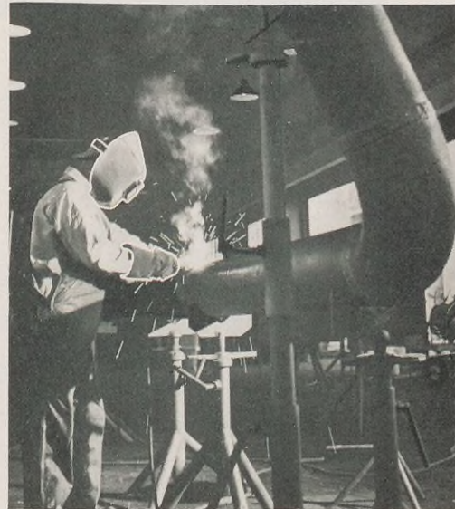
Hazard: Burns and eye injuries. Prevention: This man is doubly protected against burns by the welder's mask and gloves he wears.
