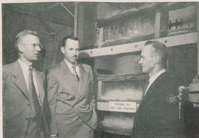
Emeryville Engineers Carl P. Strand, shown at left, and Hugh D. Guthrie, right, show Manning the experimental tray test column which was used in studying the characteristics of many different tray designs.
