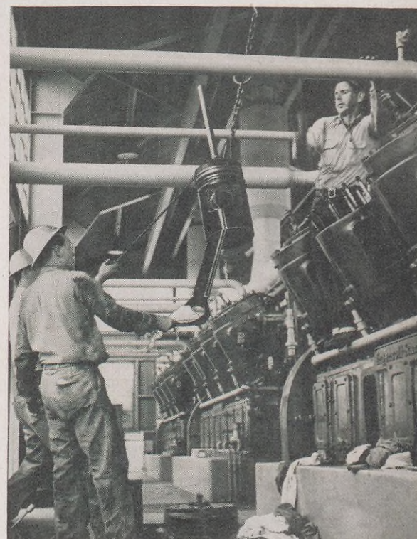
Preparing for a cleaning job, McQuade, Shackleford and Manny, above, remove a power piston from a compressor-engine at Long Beach.
