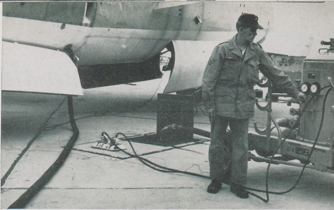
Monitoring the dials of a hose cart, Airman Second Class Donald Wallace, fuels a B-47 with JP-4 jet fuel from an underground hydrant. Aircraft are fueled when they land to prepare them for an alert or evacuation in case of an emergency.
