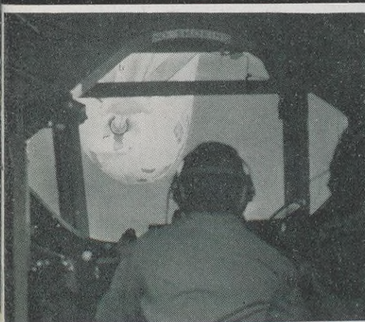
Boom operator monitors the B-47's position during contact.
