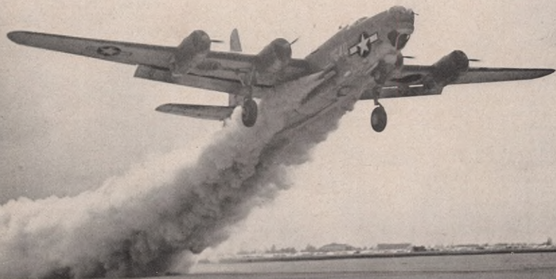
Trailing plumes of Jato exhaust, a Navy PB2Y long-range patrol aircraft is boosted into the air after a short run by the rocket action of "jet-assisted take-off" units
