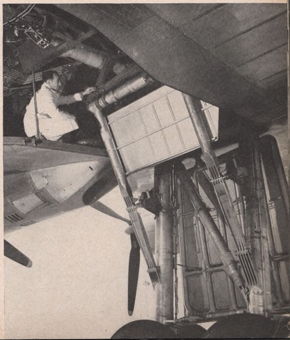
A centralized lubricating system for the Constitution's landing gear cuts lubrication time from hours to minutes
