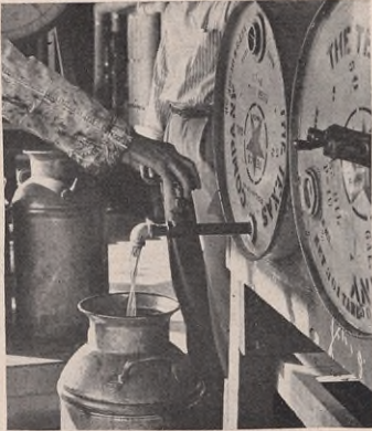
A light Texaco motor oil is measured before mixing with asphalt and an oxidant
