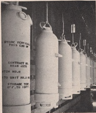
Suspended from conveyor belt, units are painted en route to shipping department
