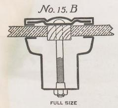
Where short lengths are required for divisions in transoms, we furnish this Bar 15-B which has the same outer member but a smaller inside member. This is somewhat lower in price than the 15-A and contains sufficient strength for the purpose intended.
