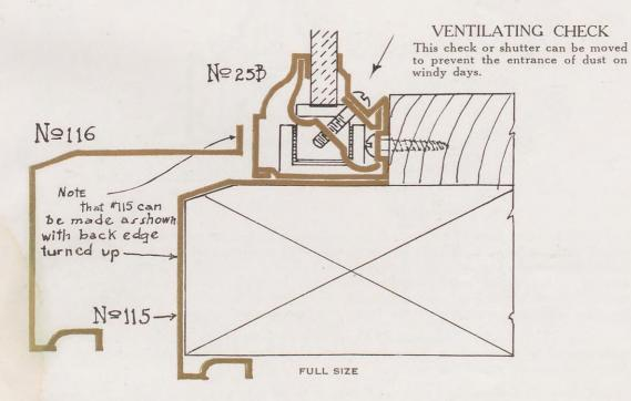
All Types of our Metal Sash embody the Ventilating and Drainage Feature.
