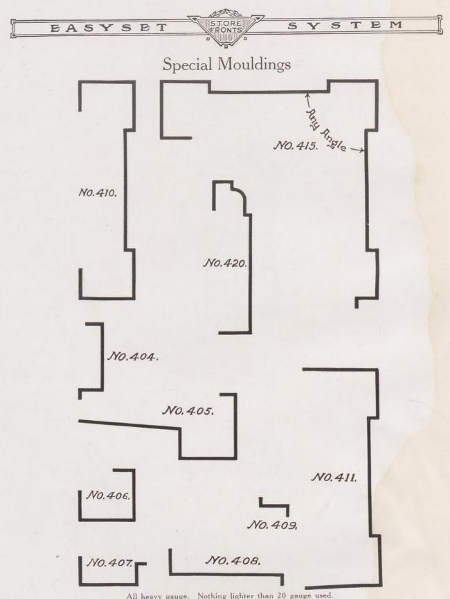
All heavy gauge. Nothing lighter than 20 gauge used. Special mouldings for Bulkheads, Transoms, Door Jambs, Etc.
