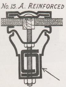
FULL SIZE Sectional View Extra Steel Reinforcing used where necessary to resist heavy pressure.
