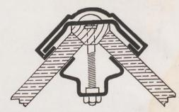
Same pattern as 4-A, but  $\frac{1}{4}$  inch larger. To be used where there is an unusual exposure to wind. Allow  $\frac{3}{8}$  inch between inner edges of glass for installation of both 4-A and 4-B.
