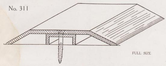
Made of No. 8 B. & S. gauge brass reinforced by short sections of steel channel. Will not rust or warp. Furnished in brass only, any length. Holes drilled at factory and screws furnished.
