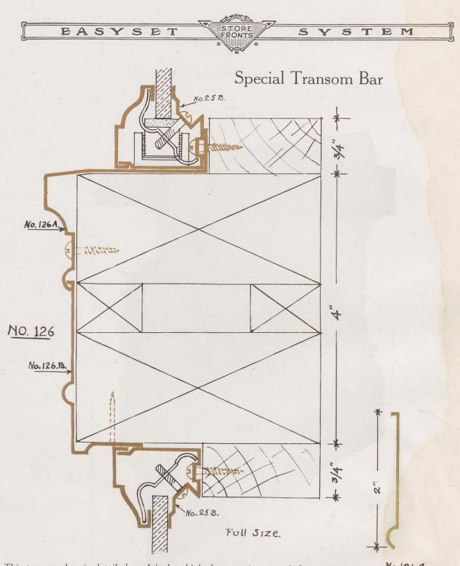
No. 126 C. To Be Used as a This transom bar is detailed as 4 inches high, but can be extended to meet requirements. HEAVY GAUGE COPPER OR BRONZE SPECIAL FINISHES Widener on No. 126 Bar. Statuary Copper, Oxidized Copper, Statuary Bronze, Nickel and Gun Metal. Other special finishes when desired.
