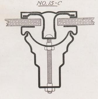
Half-inch wider than 15A. To be used with 4C Corner Bar where large glass is required, and in sections subject to high winds.
