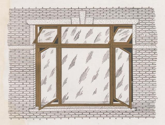
The above shows window fitted with No. 81 metal pivoted ventilating sash.
