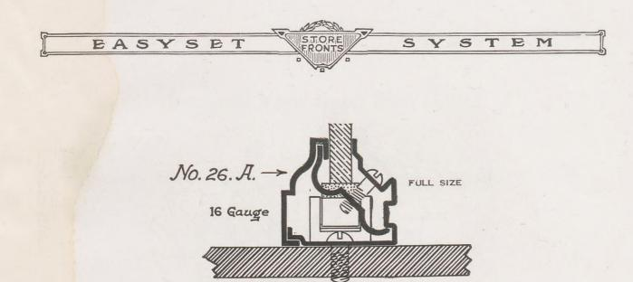
26-A. A metal Sash similar to 25-B, except that it is made of heavier metal to withstand unusual windpressure, 16-gauge copper being used. This is designed particularly to be applied to brick, stone, or steel sill, but can be attached to wood if desired, the same as design 25-B shown on opposite page.
