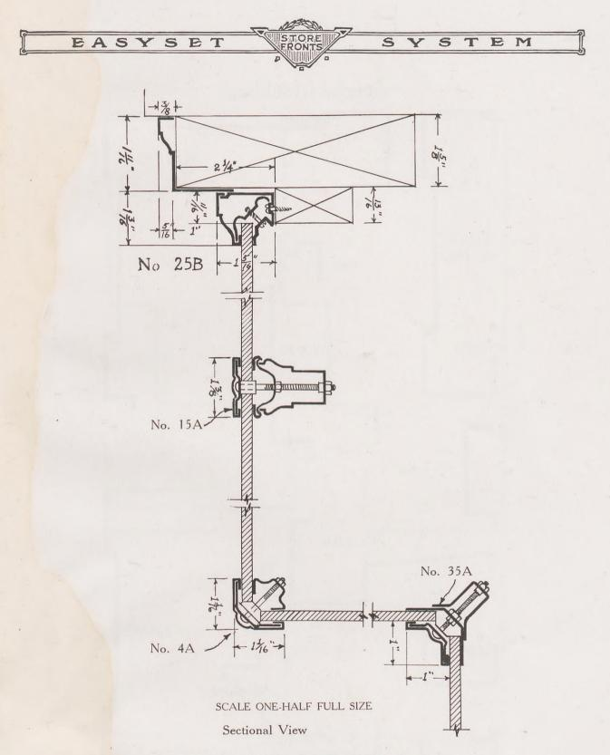
Showing Corner Bar No. 4A, Division Bar No. 15A. Reverse Angle Bar No. 35A, Metal Sash No. 25B.
