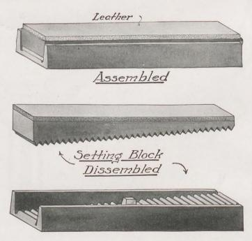
Note method of adjustment and center guard pin. This renders it impossible to throw the upper part of block off level.
