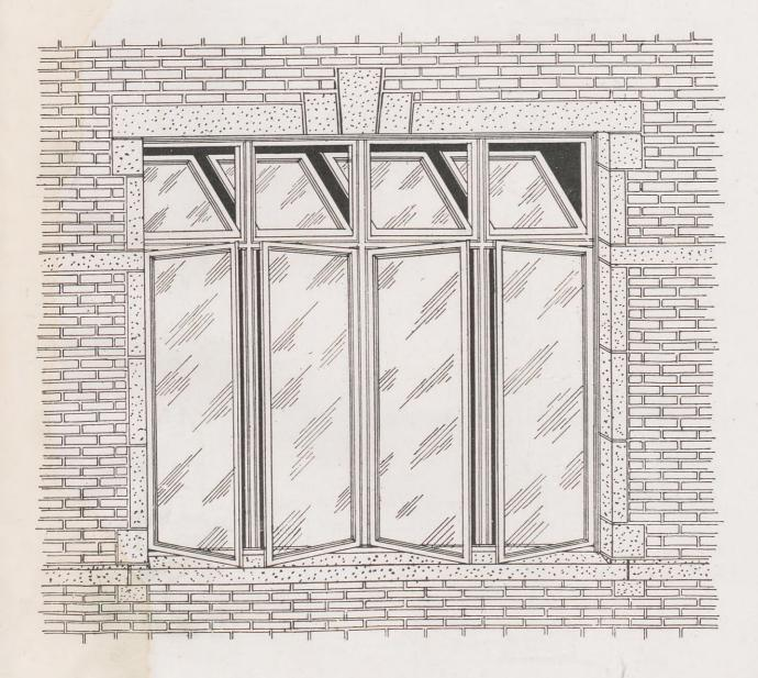
The above shows windows fitted with No. 80 metal hinged ventilating sash.
