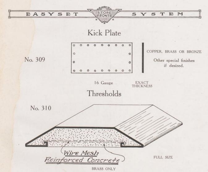
Does not swell or warp as is the case with wood filler. This threshold is fastened in place by flat head screws, countersunk, thus presenting a perfectly even surface. The necessary screw holes are drilled at our factory and sufficient screws furnished.
