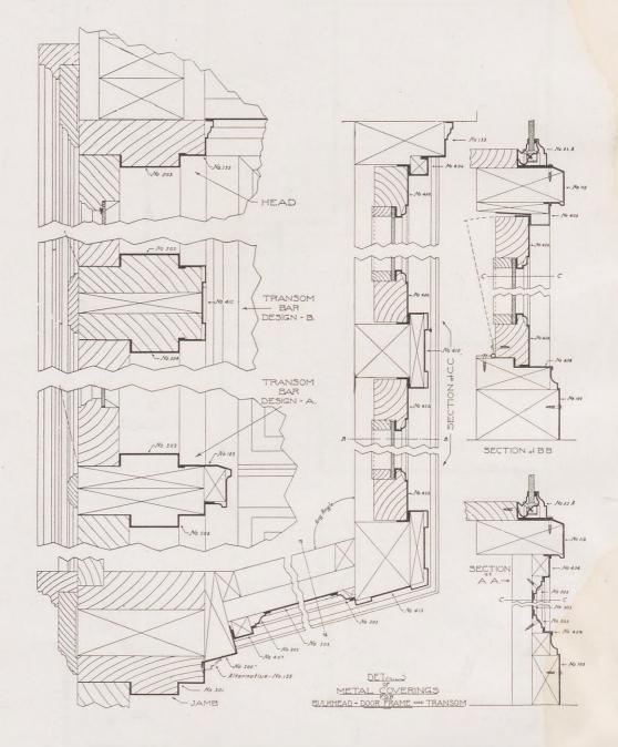
Detail showing method of application of special mouldings on preceding pages.
