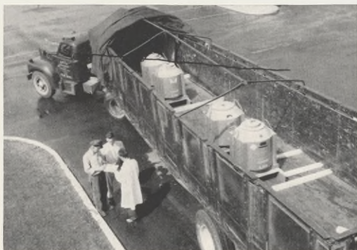
Texaco's radioactive cobalt, weighing less than 22 pounds, was trucked from Canada to Beacon in four 6,500-pound casks.
