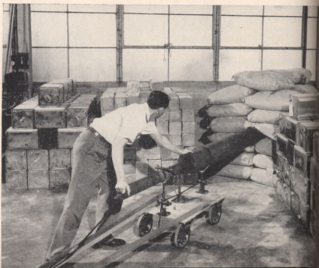
CUTTING SUBSURFACE cores is another method of learning as much as possible about underground formations. Core samples will be sent to a core laboratory to be analyzed for fluid content
