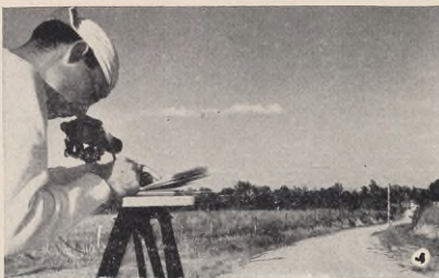
SURVEY TEAM plots site of next shot-hole a reflection seismograph party will make. Shooting is repeated along a gridwork laid out at the surface
