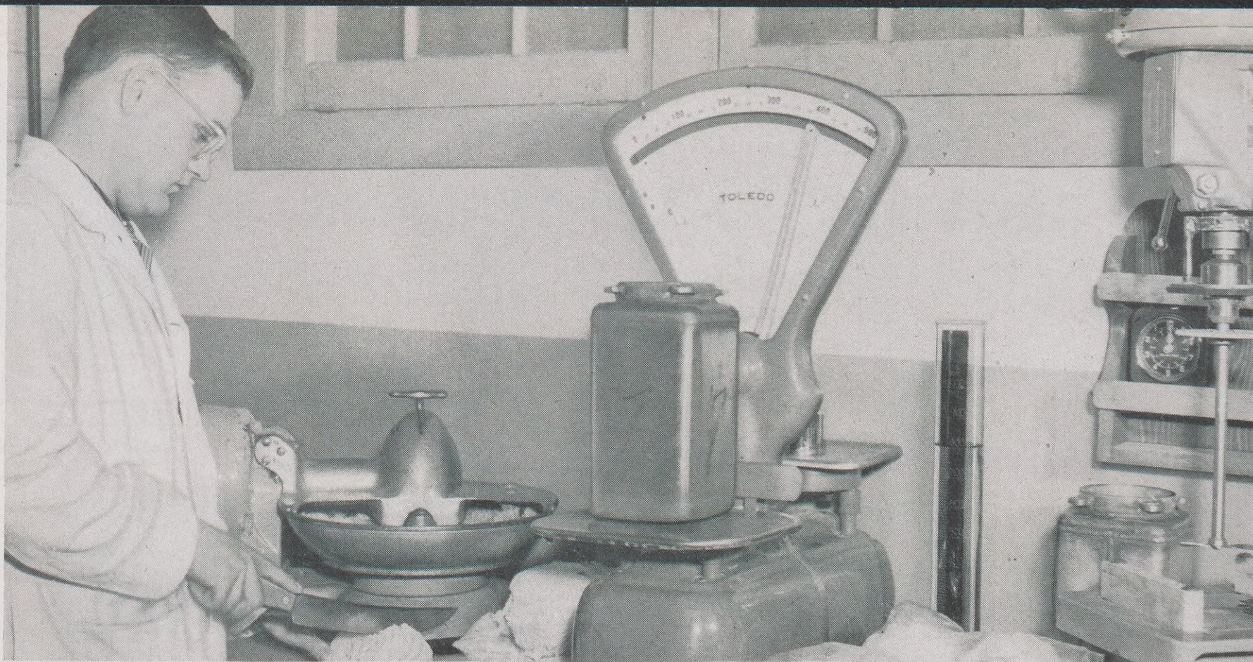
More than 1,000 residue analyses were made on 50 different crops in testing the insecticide. Here, Laboratory Assistant M. E. Coats, prepares cabbages for a test. The maximum residue permitted is one part in 1,000,000 for Phosdrin insecticide.
