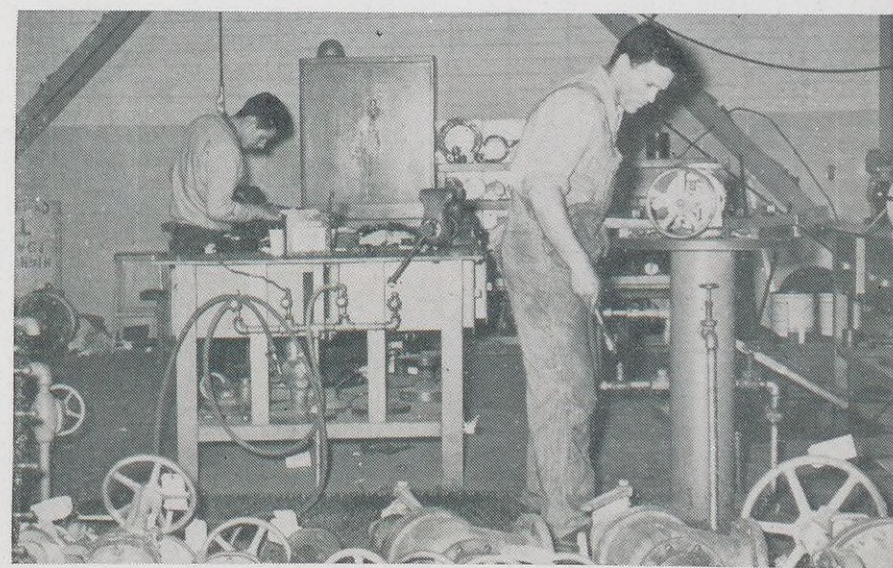
Valves galore must be checked in the turnaround. P. W. Hurlocker, Mechanic No. 1-Instrument, left, fixes instrument connection and D. C. Brown, Craft Helper-Machinist, checks one of the valves.
