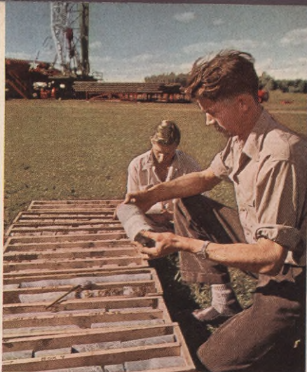
CORE SAMPLE, CUT WITH DIAMOND core bit, shows contact point where oil producing stratum and cap rock join. Core was taken from Texaco Exploration Company well being drilled at Calmar, west of Leduc. A geologist and his assistant are "logging" samples
