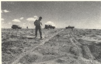
Seismic crew member lays cable used to set off explosive in the shot hole.
