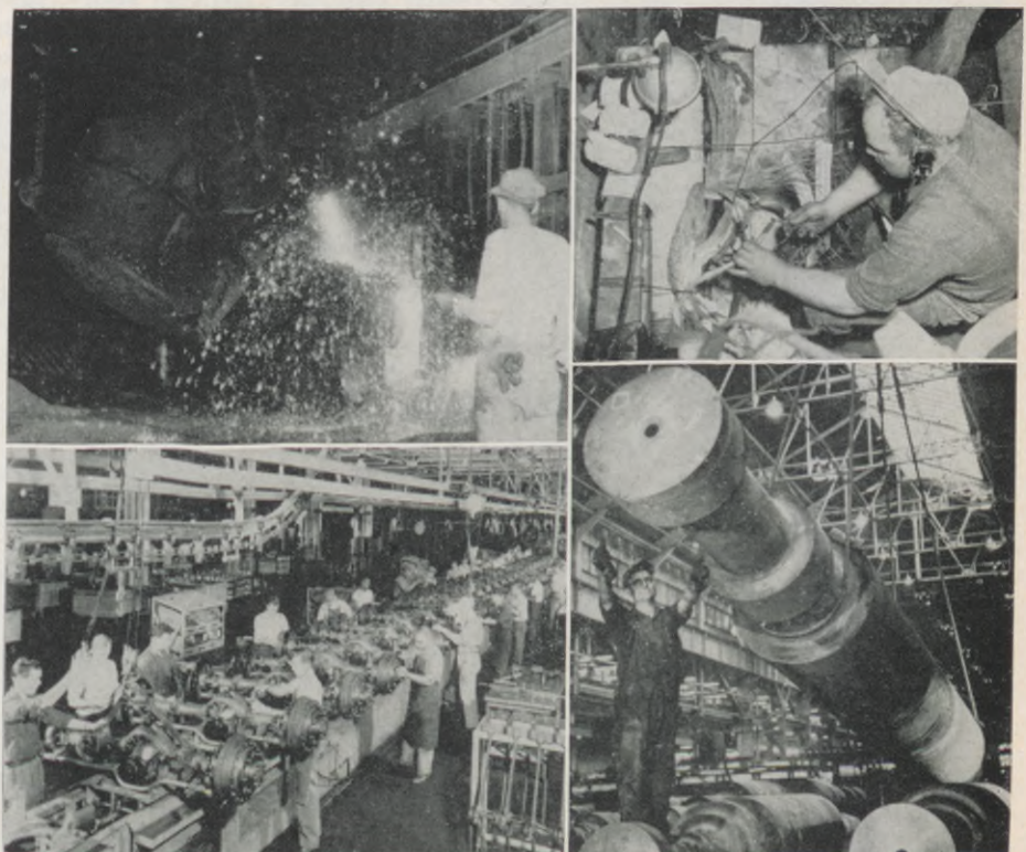
MEN AT WORK —(Top left) steelworker directs hot metal crane operator in pouring hot metal, while (top right) beneath a Chicago street a worker connects telephone wires in underground cable. (Lower left) front axles for military trucks are produced on assembly line in Cleveland plant. (Lower right) huge rough 75,000-pound forging for generator shaft of 100,000-kilowatt turbine-generator constructed at GE plant in Schenectady.
