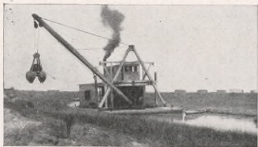
One of the six floating steel hull bucket dredges. These dredges were constructed at Port Arthur Works, and each was equipped with electric lights for working three 8-hr. shifts a day.
