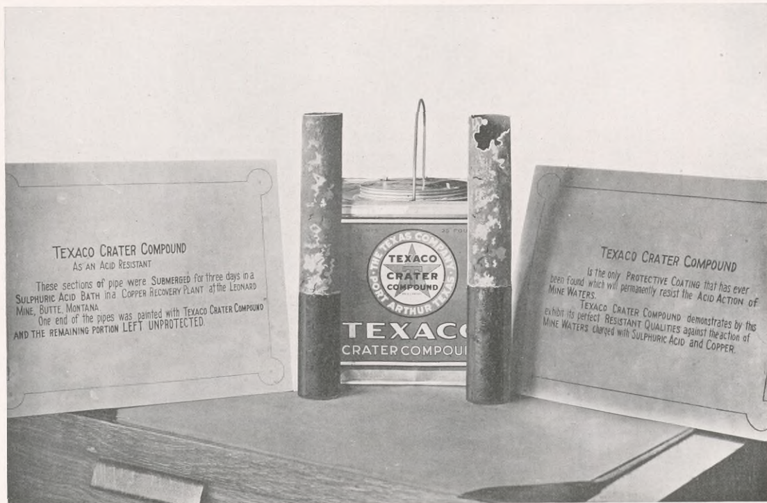
CRATER COMPOUND, ACID RESISTANT PIPE COATING—For an account of this experiment see page nine
