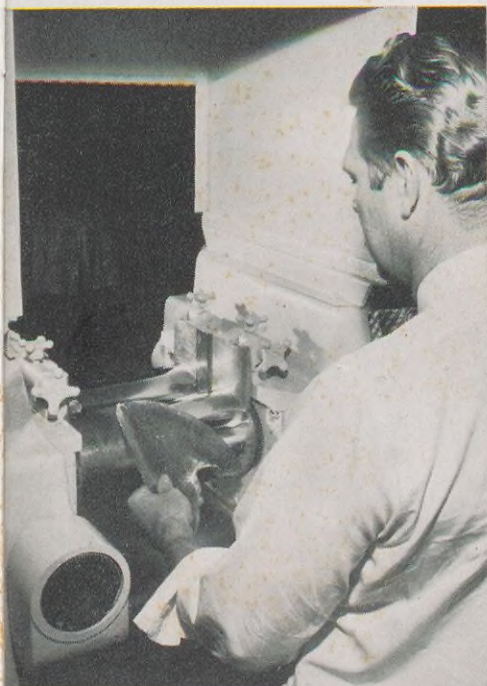
Research Chemist W. R. Hendricks runs a sample of the new product through a Torrance "rubber mill."
