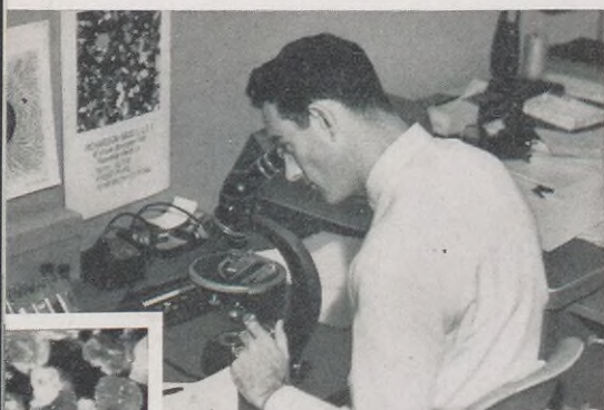
Examining a thin slice of one of the plugs is Senior Laboratory Technician A. W. Begin. He is determining in what direction the long axes of the sand grains point. At left, a photograph of the grains taken through a microscope shows that most of the long axes point in the same directions, in this case, up and down.
