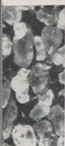
Examining a thin slice of one of the plugs is Senior Laboratory Technician A. W. Begin. He is determining in what direction the long axes of the sand grains point. At left, a photograph of the grains taken through a microscope shows that most of the long axes point in the same directions, in this case, up and down.
