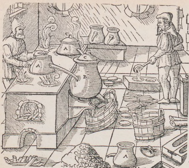
Around 1550 sulphur was refined by distillation. This picture appears in the work of Agricola, which was published early in the century.
