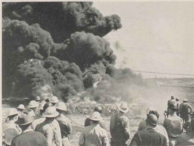
30 x 30 pit of No. 3 fuel oil topped with two barrels of gasoline one minute after ignition.
