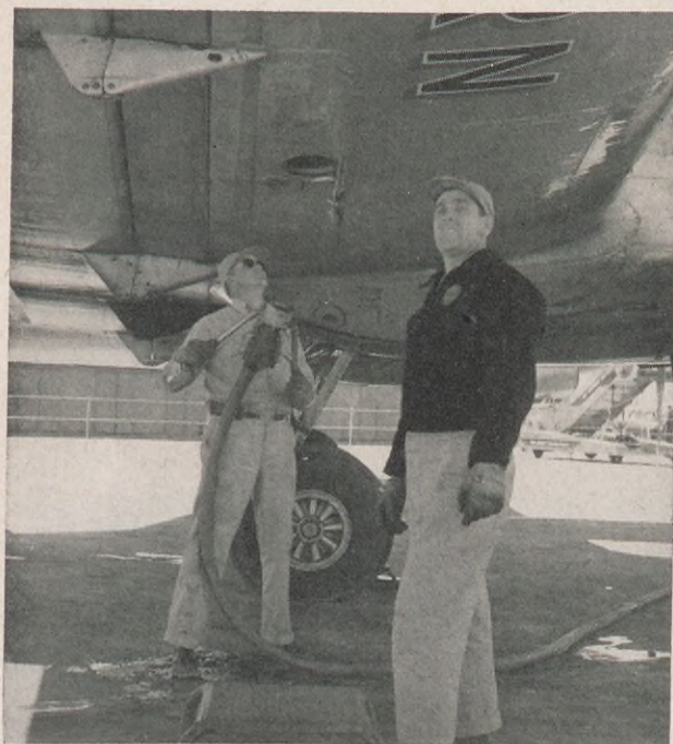
To service its account with Capital Airlines, Shell, as the Nation's first supplier of turbo-prop engine fuel to a scheduled airline, developed innovations in aircraft fueling equipment like the refueller truck, above, with special pumps for handling turbine fuel. Below, under the wing of an Eastern Air Lines Silver Falcon passenger liner, a man holds a special under-wing fueling attachment, pioneered earlier by Shell, which facilitates the job.
