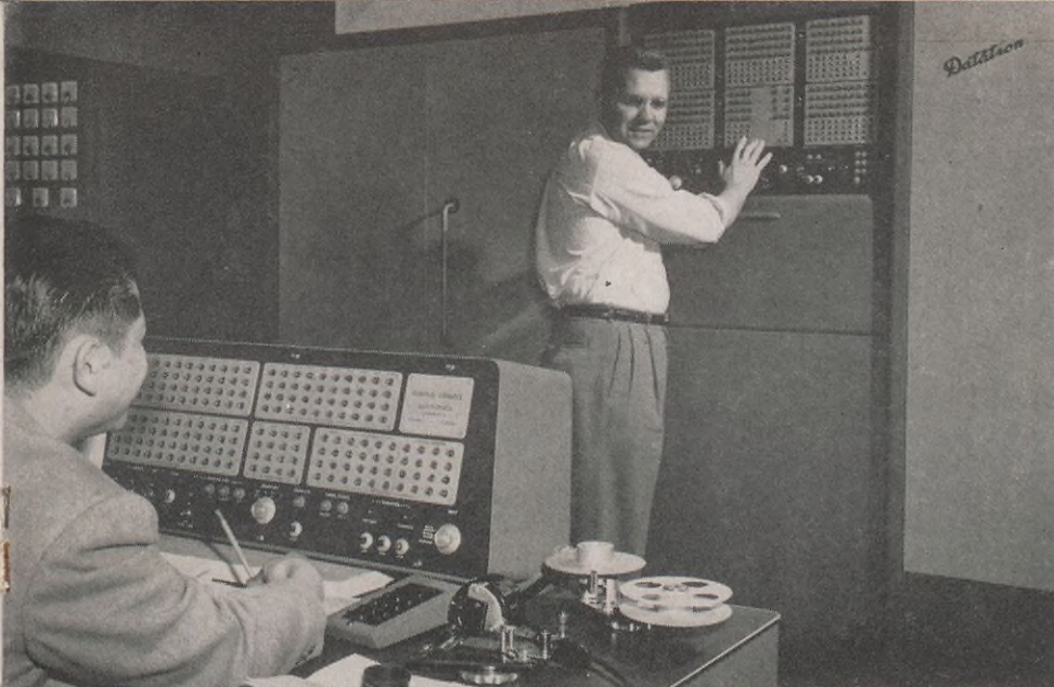
An ElectroData computer installed at Emeryville during 1955 helps to reduce the time between basic research and commercial production by quickly solving complex mathematical problems. Above, W. Yuen, left, and F. G. Stockton run a problem through the computer.
