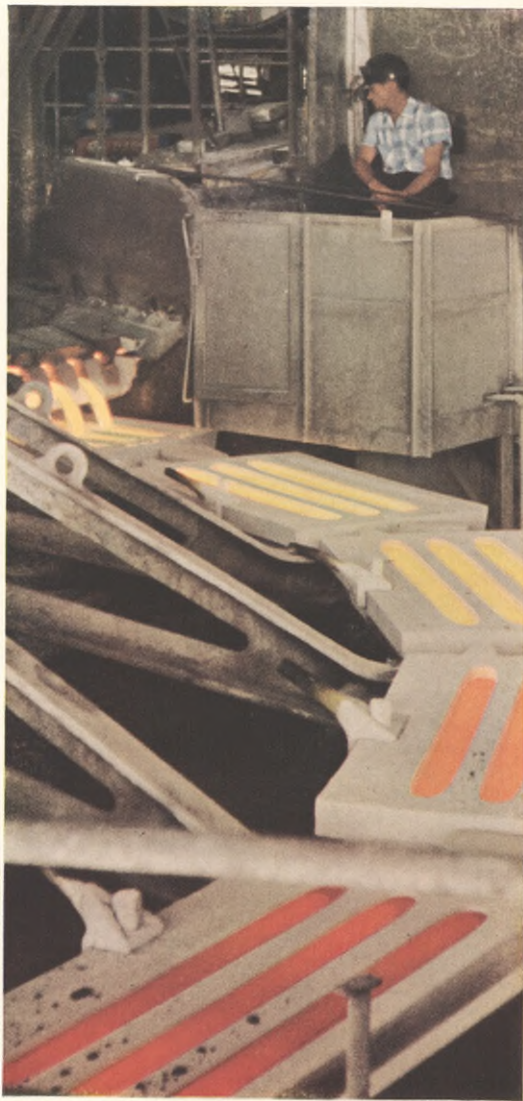
On a smelter converter floor, facing page, a workman swings into position the massive arms that carry ladles of molten copper. An overhead crane carries the metal to nearby casting wheel, above.
