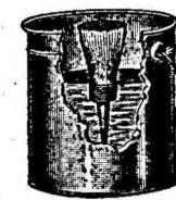
A good method for preserving used paint brushes is to suspend them in water by running a wire through a hole in the handle of the brush and allow the water to cover the bristles only. Another way is to drive nails through the side of a wood bucket and suspend the brushes on the nails (see illustration.)
