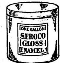
Then with a 2 or 2½-inch varnish brush apply the enamel, commencing at the top and work downwards. Spread on an even coat and not too sparingly; put on plenty of it, but not enough to cause it to run. Do not brush out as you would in painting; as few strokes as possible will make a better finish. Should the enamel be very thick, thin with turpentine, but do not add more than is necessary.
