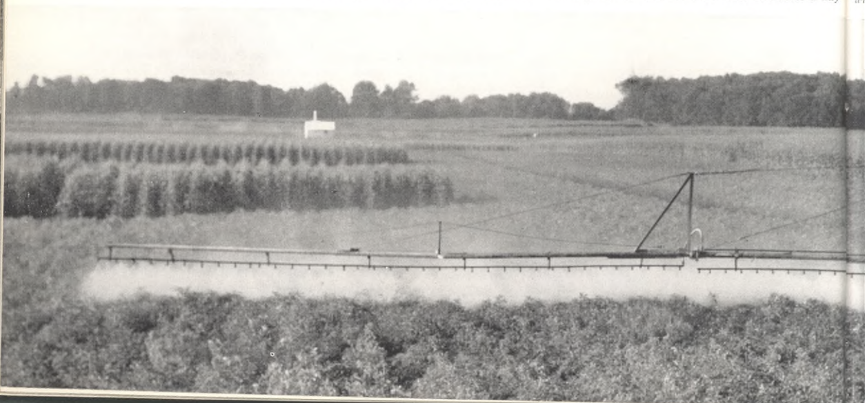
Gigantic boom of specially built crop sprayer stretches for 75 feet across an onion field; one man can cover over 150 acres a day
