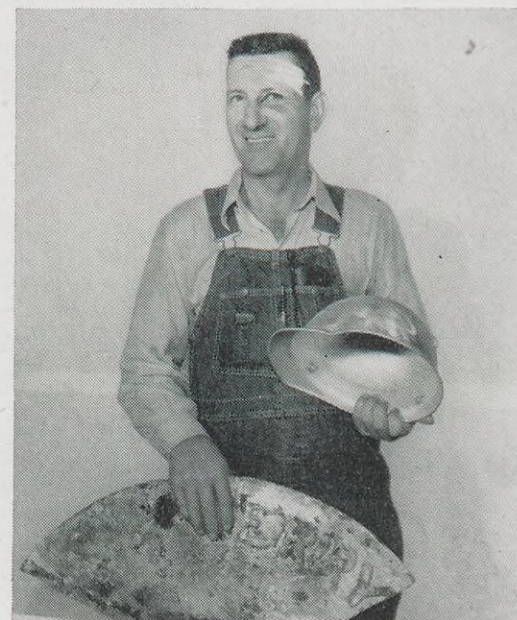
An exploding turbine case threw a 38-pound fragment at Pipefitter E. W. Bryant's head at the Wood River Refinery. He suffered a slight cut.
