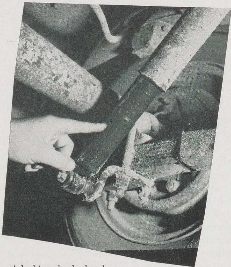
A leaking shock absorber, often not noticed until the car is on a lube rack, can make the car shimmy at high speed.
