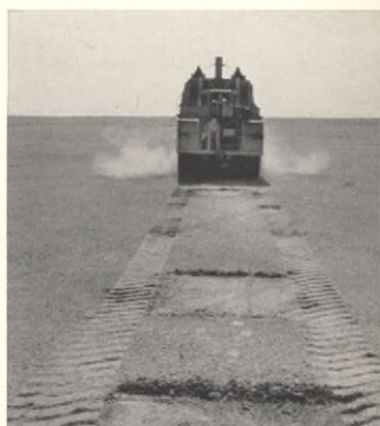
"Stomper" pounds desert, creates seismic vibrations.
