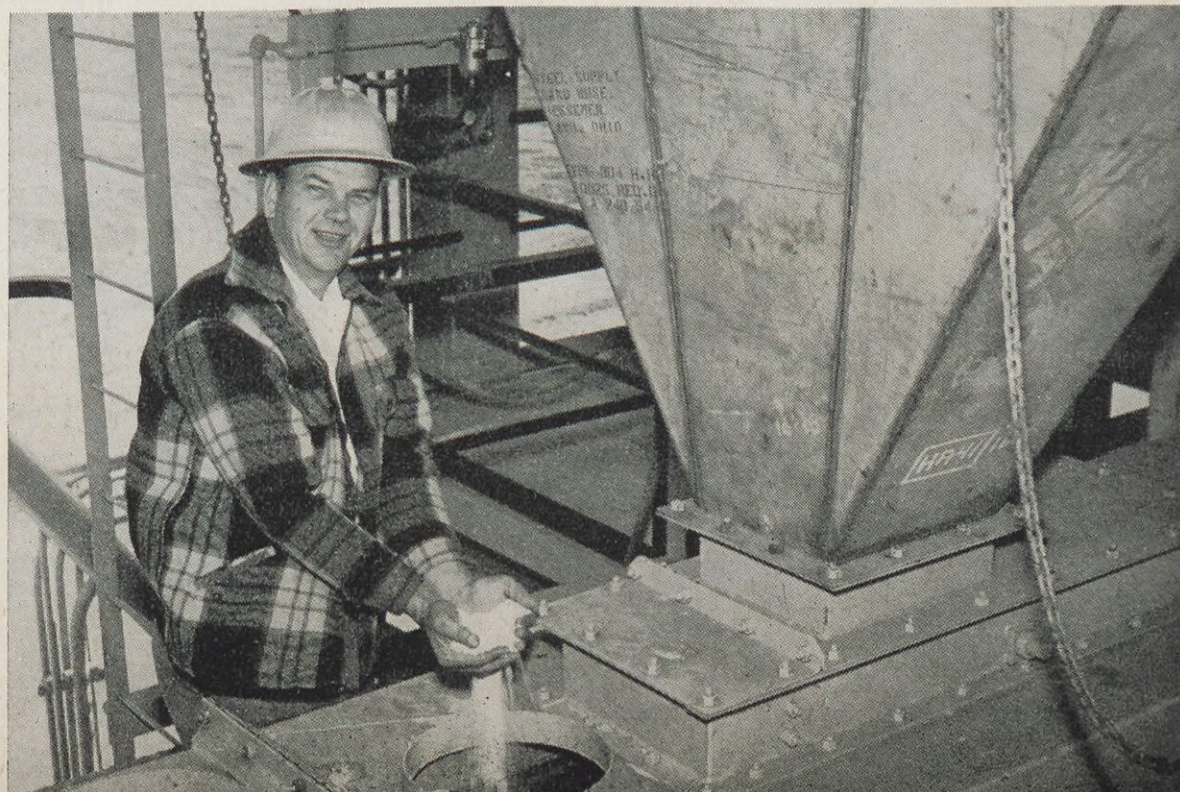
Loading Foreman L. R. Wallace inspects urea prills as the product moves from a hopper to be packaged in heavy paper bags.
