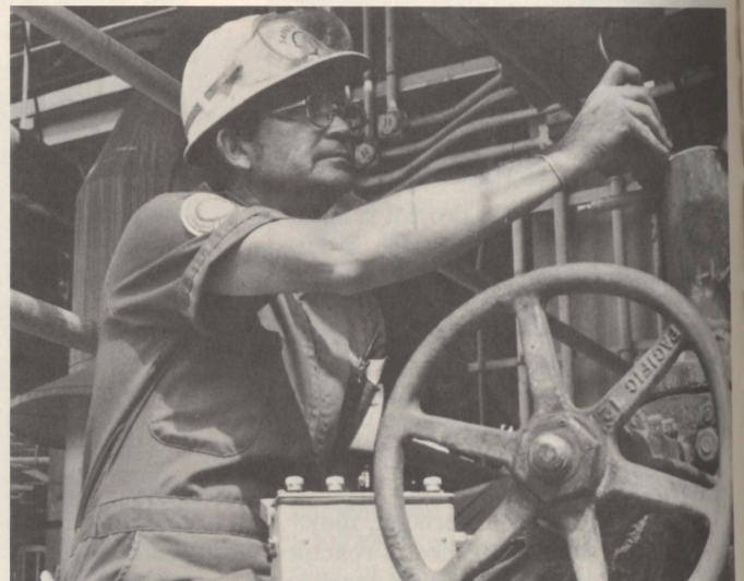
Herb Ely, a Safety inspector, uses a combustibles indicator to check a line for potential flammable concentrations of hydrocarbon vapors.
