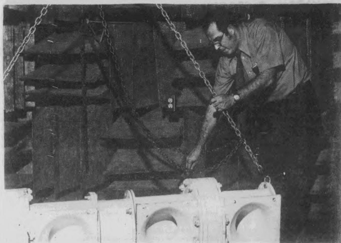
DR. WILLIAM RYAN of the U.S. Coast Guard headquarters in Washington, D.C., Thursday in the anachroic chamber on the first floor of the Engineering Building, prepare a fog horn for acoustical tests.
