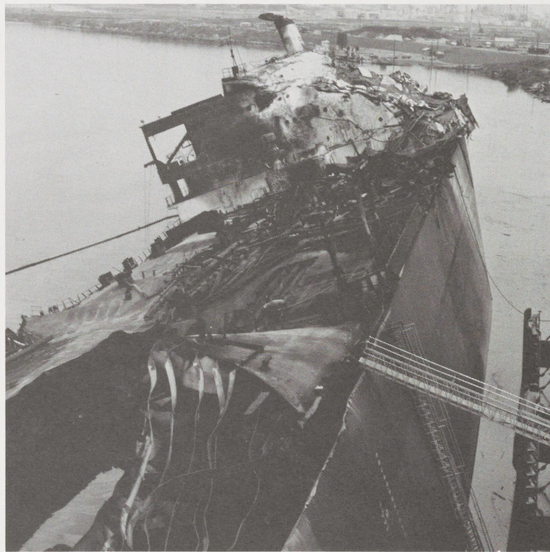
The scarred hull of the Chevron Hawaii gave evidence to the devastation of the explosion and fire that engulfed the ship. But the jumbo tanker, written off as a total loss, had more sailing to do.
