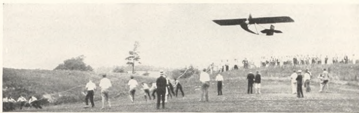
Catapulting a "Primary" Glider into the Air With Elastic Rope
